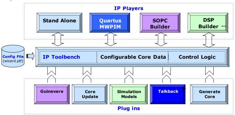
The IP Toolbench framework is built on central configuration file (wizard.ptf) that defines the core, initializes IP Toolbench configurable core data, and specifies which plug-ins should be loaded for this core. Currently, this configuration file is written in PTF format, but we plan on eventually migrating this to XML using Corespec.
