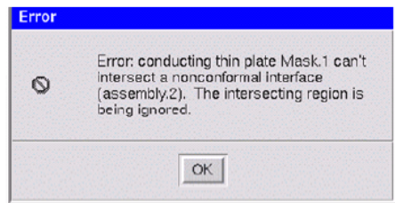
Figure 7.2: Thin Conducting Plate Intersecting the Non-Conformal Boundary
