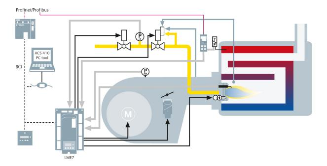
The diagram shows the full scope of functions of the LME75/LME76. The actual functions are to be determined based on the respective execution or configuration.
