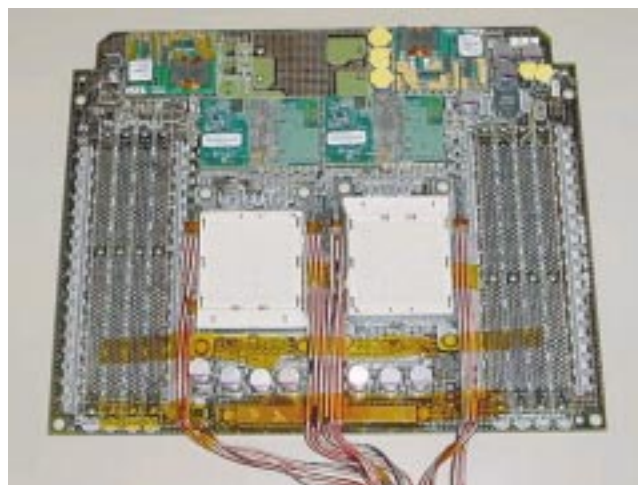
Figure 3-3 Board with SMT Components Only (After SMT Reflow) Example 1
