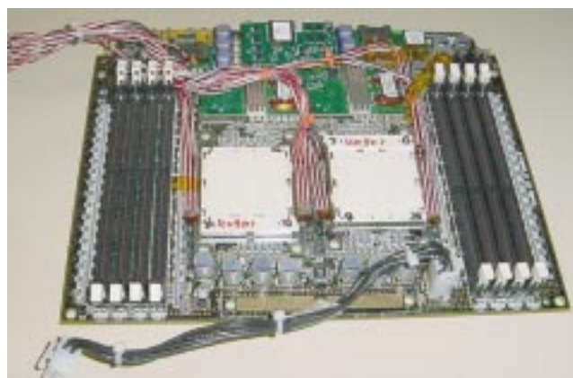
Figure 3-5 Board with Both SMT and Through-Hole Components (After Wave Solder)
