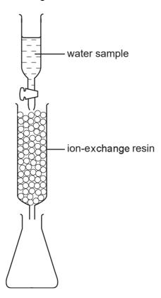
A 50 cm $^3$  sample of water containing dissolved calcium sulphate was passed through the ion-exchange resin. Each calcium ion in the sample was exchanged for two hydrogen ions. The resulting acidic solution collected in the flask required 25 cm $^3$  of 1.0  $\times$  10 $^{-2}$  mol dm $^{-3}$  potassium hydroxide for complete neutralisation.
