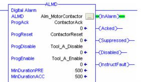
The instructions are defined in RSLogix 5000 as an alarm datatype and configured using property panels. All necessary alarm properties that previously had to be defined and maintained in the HMI, such as alarm limit and current status, are now defined and maintained in the controller as tag parameters.
