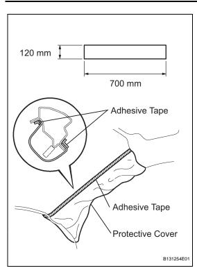
(5) Thoroughly cover the airbag with cloth or nylon of 700 mm (27.56 in.) x 120 mm (4.72 in.) and fix the ends of the cover with adhesive tape, as shown in the illustration.
