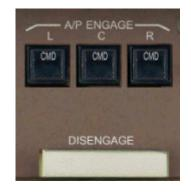
Each FCC has an independent power source when activated will provide flight control input directly to the flight controls through three independent hydraulic systems. As such, each FCC can be allowed to have full independent control of all aircraft flight control surfaces, or multiple FCCs can be operated in tandem to provide full fail-safe operation for coupled approaches and autoland.
