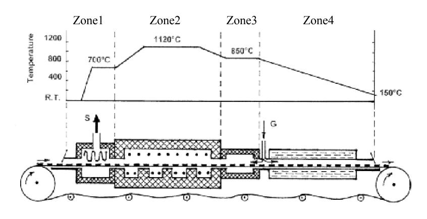
Zone1 = Burning-off Lub, 2 = Sintering, 3 = Re-carburizing, 4 = Cooling G = Gas inlet, S = Smoke and gas outlet
