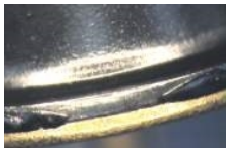
To-Can封盖焊带缺陷
