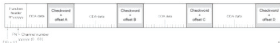
Figure 3 – 56-bit or 7-byte ODA group type C structure
