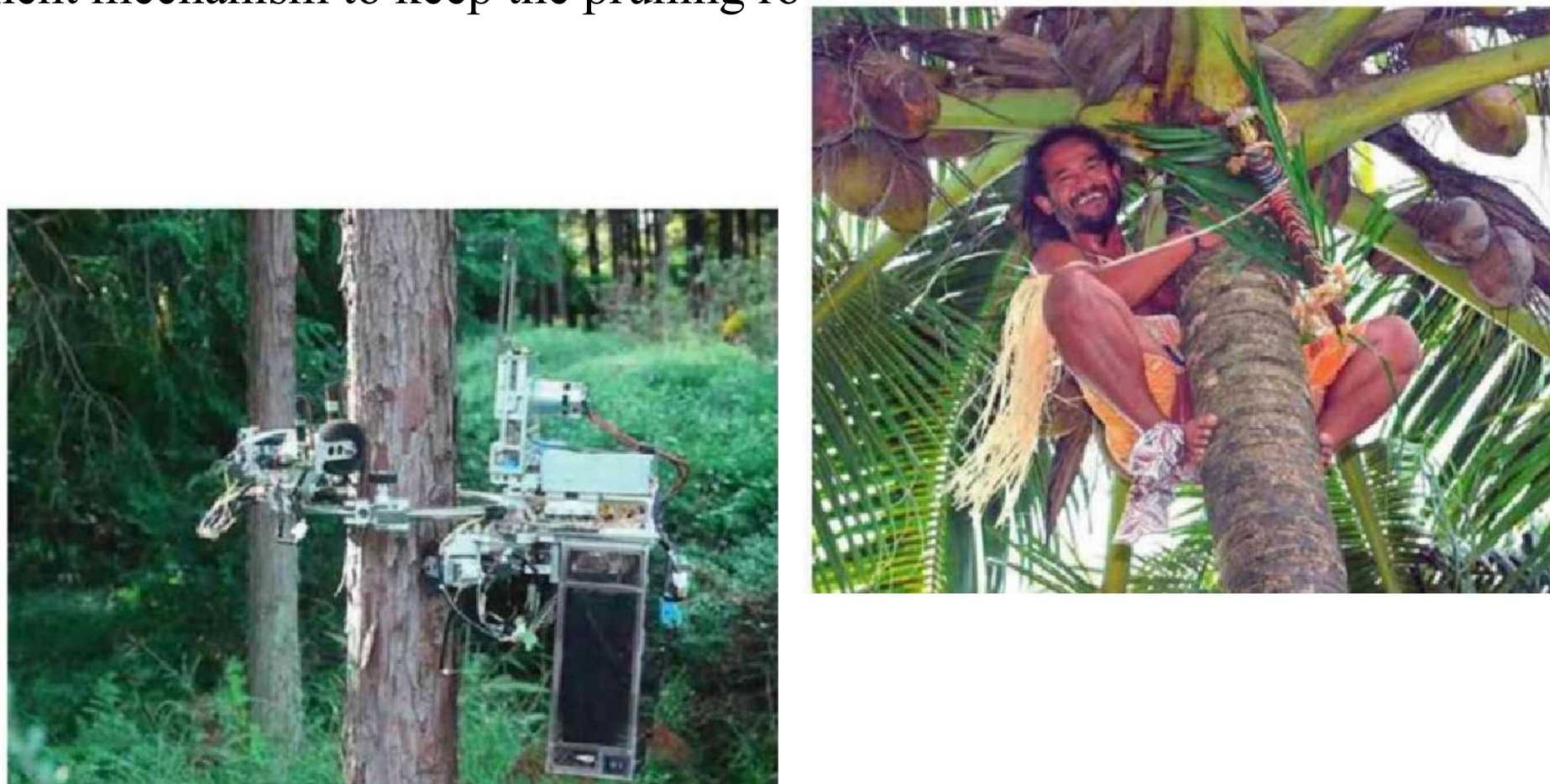
Figure 14.8 On the left, the pruning robot adjusts its posture to stay on the tree using only its weight. The same technique is used for centuries by coconut tree climbers.
