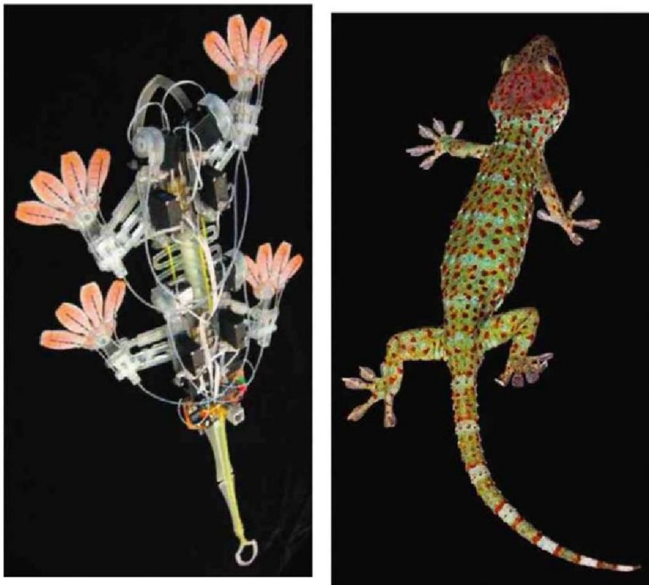
Figure 14.6 On the left is the StickyBot and on the right is an underside view of a Gecko showing the details of its fingers.
