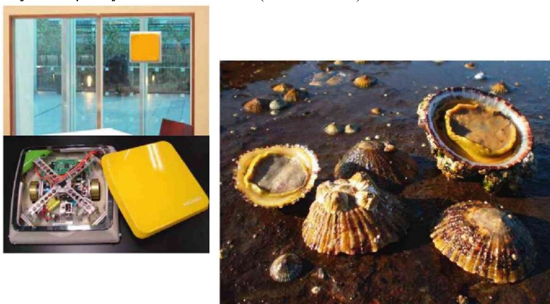
Figure 14.4 On the left, the WallWalker window cleaning climbing robot. On the right, an example of natural wet adhesion with suction used by limpets (photo courtesy of Jay from Naturebum).
