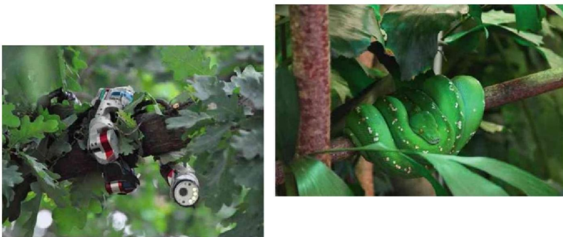
Figure 14.10 The CMU unified snake robot climbing a tree. This locomotion concept draws inspiration from snakes.
