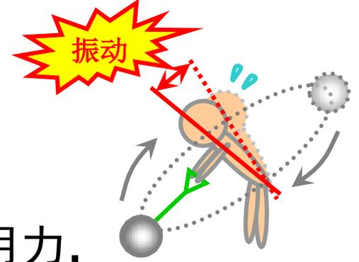
$$F(\text{离心力}) = m(\text{分铜重量}) \times \omega^2(\text{回转数}) \times r(\text{重心距离})$$
