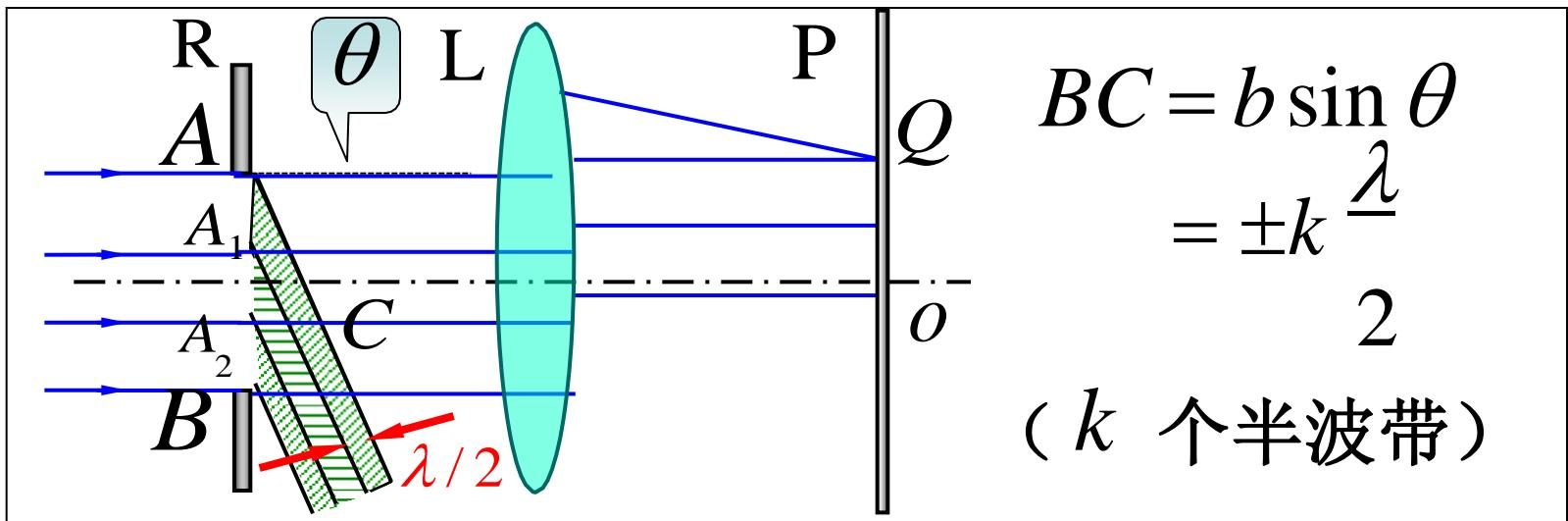
$$\left\{ \begin{array}{l} b \sin \theta = 0 \quad \text{中央明纹中心} \\ b \sin \theta = \pm 2k \frac{\lambda}{2} = \pm k\lambda \quad \text{干涉相消(暗纹)} \\ b \sin \theta = \pm (2k+1) \frac{\lambda}{2} \quad \text{干涉加强(明纹)} \\ b \sin \theta \neq k \frac{\lambda}{2} \quad (\text{介于明暗之间}) \quad (k = 1, 2, 3, \dots) \end{array} \right.$$
