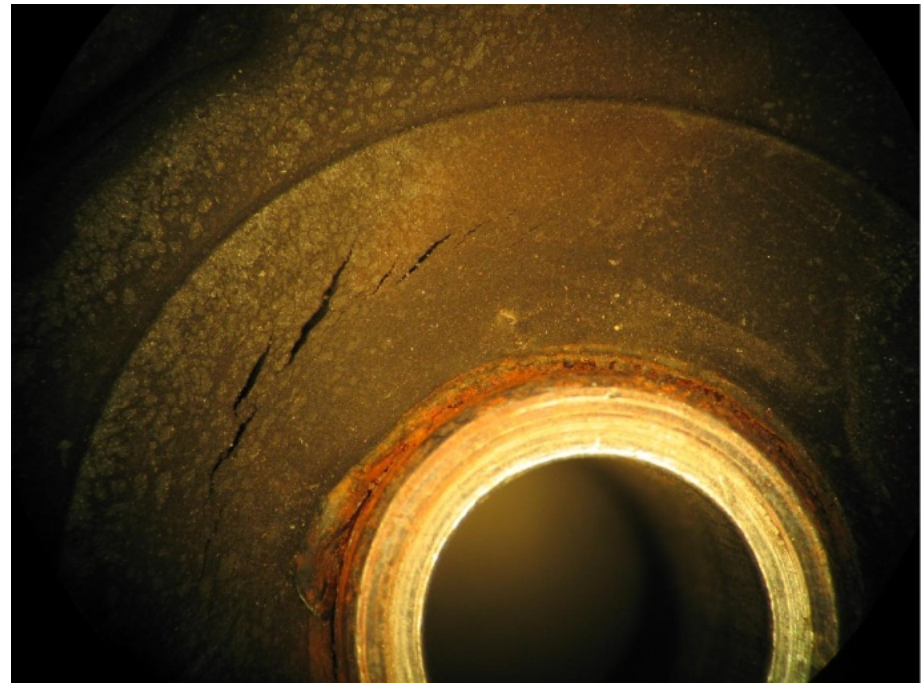
Propeller shaft disc Component failure
