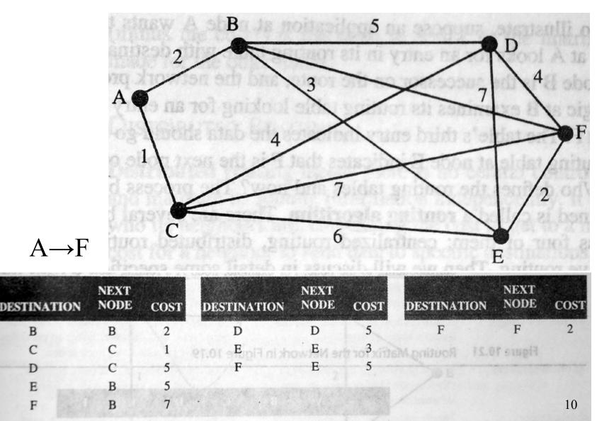
(a) Partial routing table for node A (b) Partial routing table for node B (c) Partial routing table for node E
