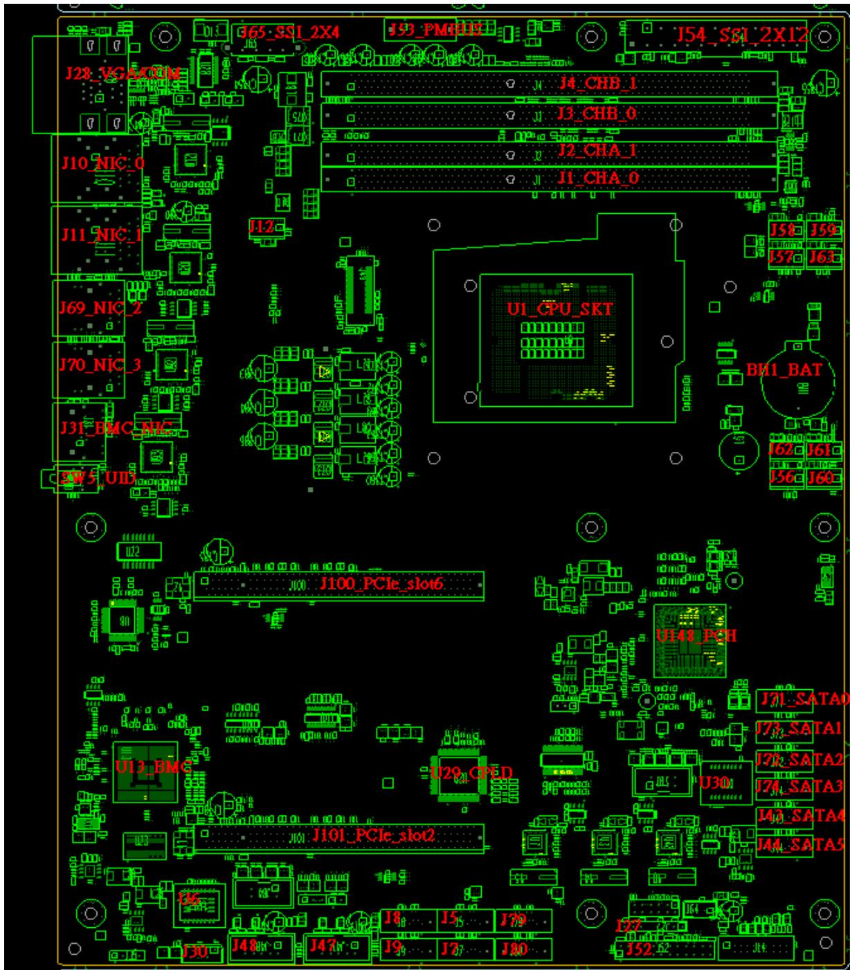
Figure .1 Placements on Motherboard
